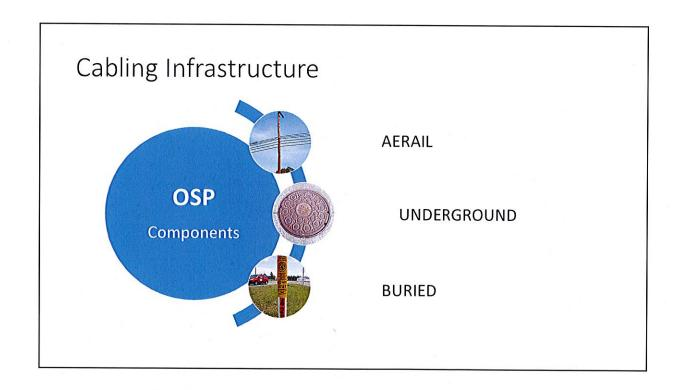
AERAIL: Involves the use of utility poles, either sole owned power, or communication poles, and or joint use poles (multiple owners), along with communication towers.
